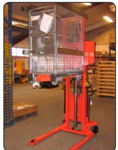
Logiflex ELF with Rotator used at the Swedish postal services for emptying letter containers into sorting machines.
