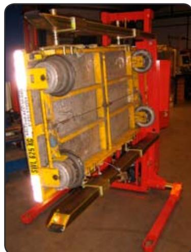
Logiflex straddle stacker with Rotator for the handling of small railway trolleys when carrying through service and repair.
