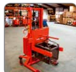
Logiflex with side-tilting forks and spear to carry and turn wire boxes.
