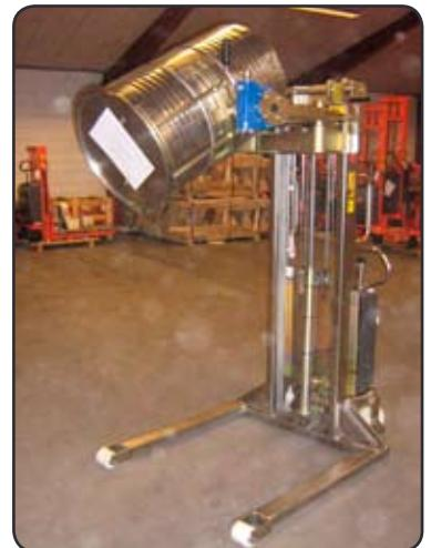
Stainless stacker with drum turner for lifting and emptying drums.
