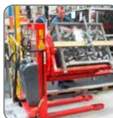
The Rotator is here used in the component industry.
