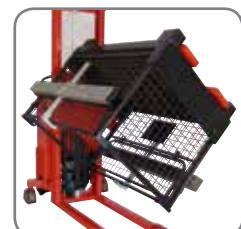
The Rotator can turn a box 180° to empty it fully, when equipped with box holders with clamps.
