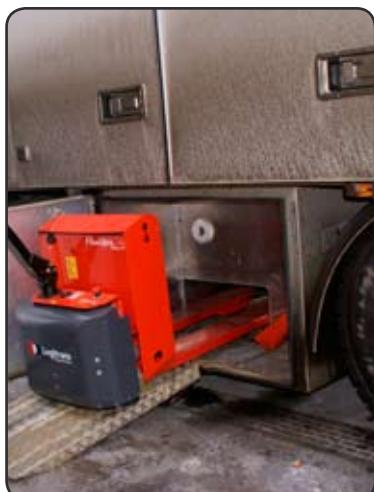
A special low construction makes it possible to place a Panther Maxi AC in a transport box under the lorry during transport. This gives room for two more pallets in the lorry.
