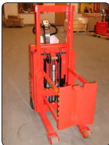
SELF Maxi with special drum lifter. One of the handle grips of the drum is used to fix the drum.
