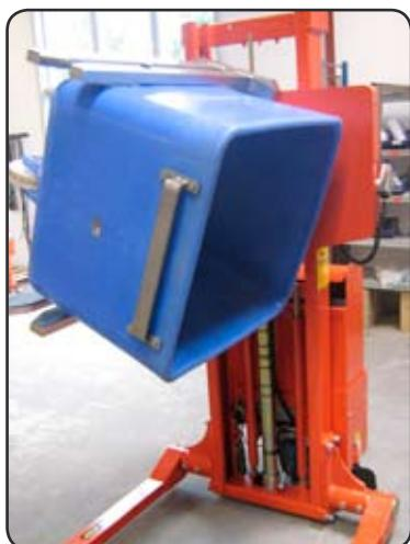
SELFS with Rotator for the handling of Vemag-containers. Used at a marzipan factory in Denmark.
