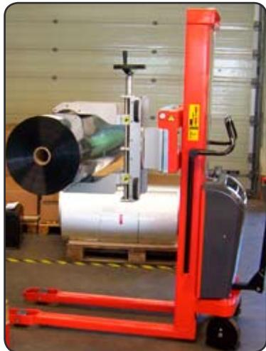
Special reel clamp for very smooth and 200 kg heavy reels of anti-magnetic folio for electronic parts.
